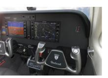
Garmin® GI 275 Electronic Standby, and the Garmin® GMC 707 Autopilot Control Panel. Electronic Stability and Protection (ESP) and Underspeed Protection (USP), carbon monoxide (CO) detector and multiple cockpit dual USB ports come standard.
